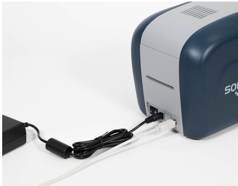
Figure 8 SOLID-310S Connection of power and USB cable
